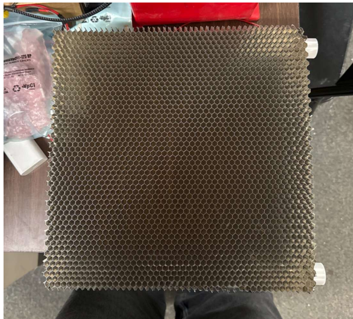
Figure: Aluminum honeycomb flow straightener (1/4" hex cells, 1" thick)
