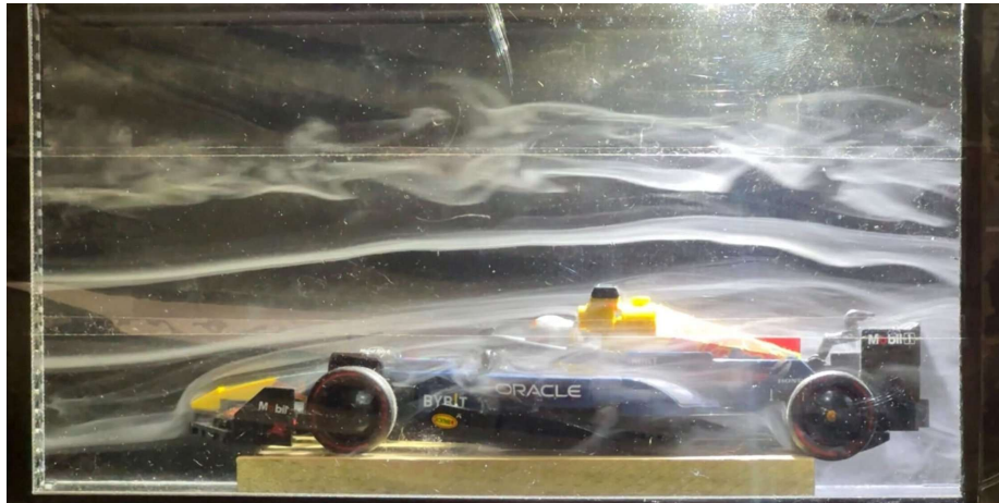
Figure: Laminar smoke flow over scale model car with honeycomb installed (12V, 0.7–0.8A)
