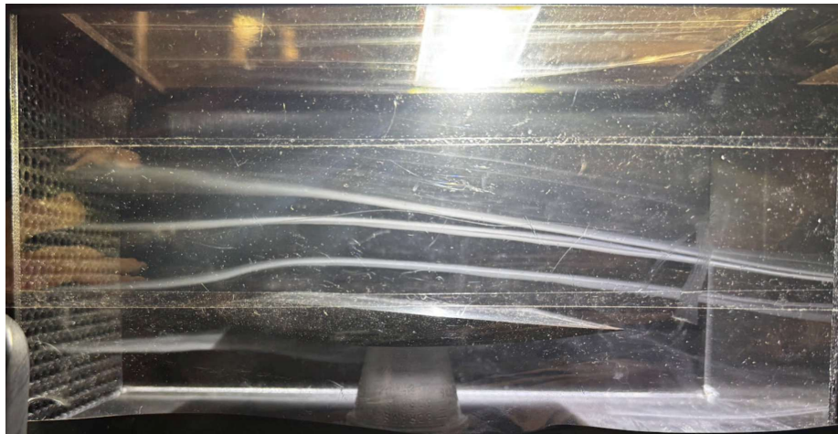
Figure: Laminar smoke flow over airfoil — cleanest flow visualization result achieved
